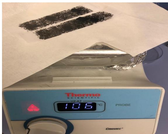
**Figure 3.7:** Microscope glass slides pushing keeping scotch tape with 300nm  $\text{SiO}_2/\text{Si}$ -substrate on a hot plate
