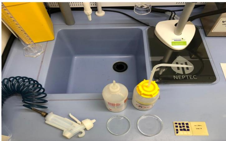
**Figure 3.1:** From left to right: Pressurized  $N_2$  gun, Acetone and Isopropanol, cleaned silicon chips
