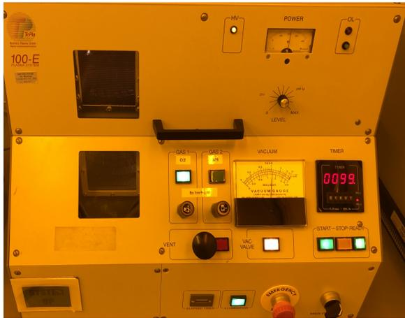
**Figure 3.2:** Giga-Etch 100-E Plasma Etcher while doing  $\text{O}_2$  Plasma at 285W, 0.5mBar for 3 minutes
