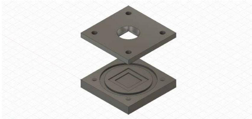
**Figure 4.11:** 3D model of the sample holder using to protect patterned front side during wet etching.
