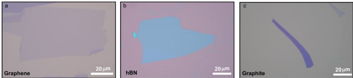
Figure 3.1.1: Flake Selection. (a) A suitable graphene flake should be at least twice as large as the desired device size, with an aspect ratio of 2:1. (b) The hBN flake should be free of tape residues, step-terraces, defects, or folds. The thickness should be around 10-15 nm, and a sharp edge is needed to lock the graphene. (c) A suitable graphite gate is \sim 2-4 nm thick, 3-7 \mu m wide and 10-15 \mu m long.
