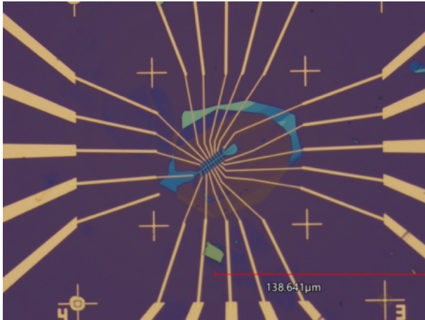
FIGURE 24: Optical microscope picture (x50) of the device after the evaporation process. One can see the freshly evaporated Cr/Au electrodes connecting the device to the pre-patterned electrodes.
