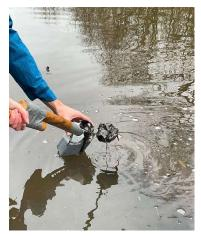
How to collect samples? We have never done it yet, but I will try to explain it briefly. Samples are taken from lakes or small streams. Using a kitchen ladle, possibly attached to a pole or broomstick, you can collect some mud from the top layer at the bottom of the lake/stream, not too far
