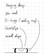
Brian has drawn it. You need a microscope slide and coverslip. One drop is put on the coverslip. Then you set the O-ring (just something so that there is space for the drop between the glasses) on the coverslip, then the slide. You take both and turn it upside-down,
