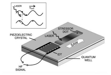
Schematic sketch of a SAW sample for the acoustically driven transport of electron hole pairs. The material of the system may be, for example, GaAs for the piezoelectric crystal, InGaAs for the quantum well, and InP for the stressor. The inset depicts the storage of optically generated excitons in the potential of the surface acoustic wave. These spatially separated excitons may recombine at the location of the quantum dot, given rise for the generation of single photons.
