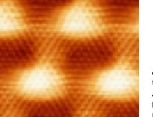
Atomically resolved image of the graphene overlayer. The image shows three different levels of apparent heights, namely four bright maxima, a dark minimum in the center between the three maxima on the right hand side, and a less dark minimum between the three maxima on the left hand side.  $50 \text{ Å} \times 40 \text{ Å}$ , It = 1 nA,  $V_{\text{sample}} = -0.05 \text{ V}$ .
